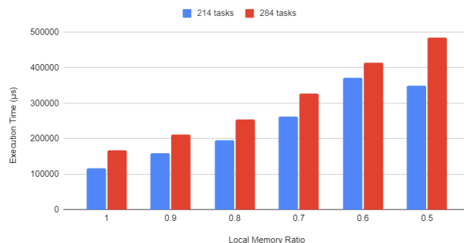
Figure 4. Runtime of the molecular design benchmark with 16 molecules simulated. Times are averaged over 10 runs with different local-remote memory ratios.
