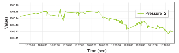
Figure 5. Time series plot in Grafana dashboard for measured pressure at Location 2 over time (y-axis: millibars, x-axis: timestamp).
