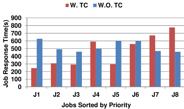
Figure 14. Job Response Time Distribution [Test Set: Benchmark=Terasort; #Nodes = 8; Job Size = 4096M] [smaller Job ID implies higher priority]
