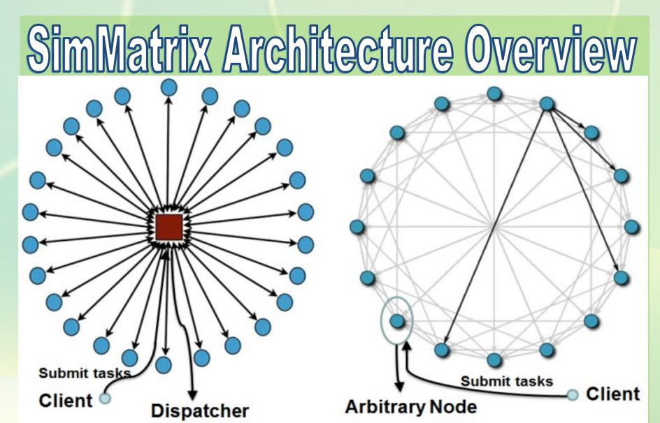
The left part is the centralized scheduling with a single dispatcher connecting all nodes; the right part is the homogeneous distributed topology with each node having the same number of cores and neighbors
