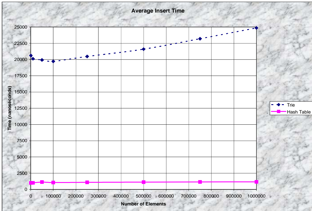
Figure 4: Average Insert Time in nanoseconds between the trie and the hash table
