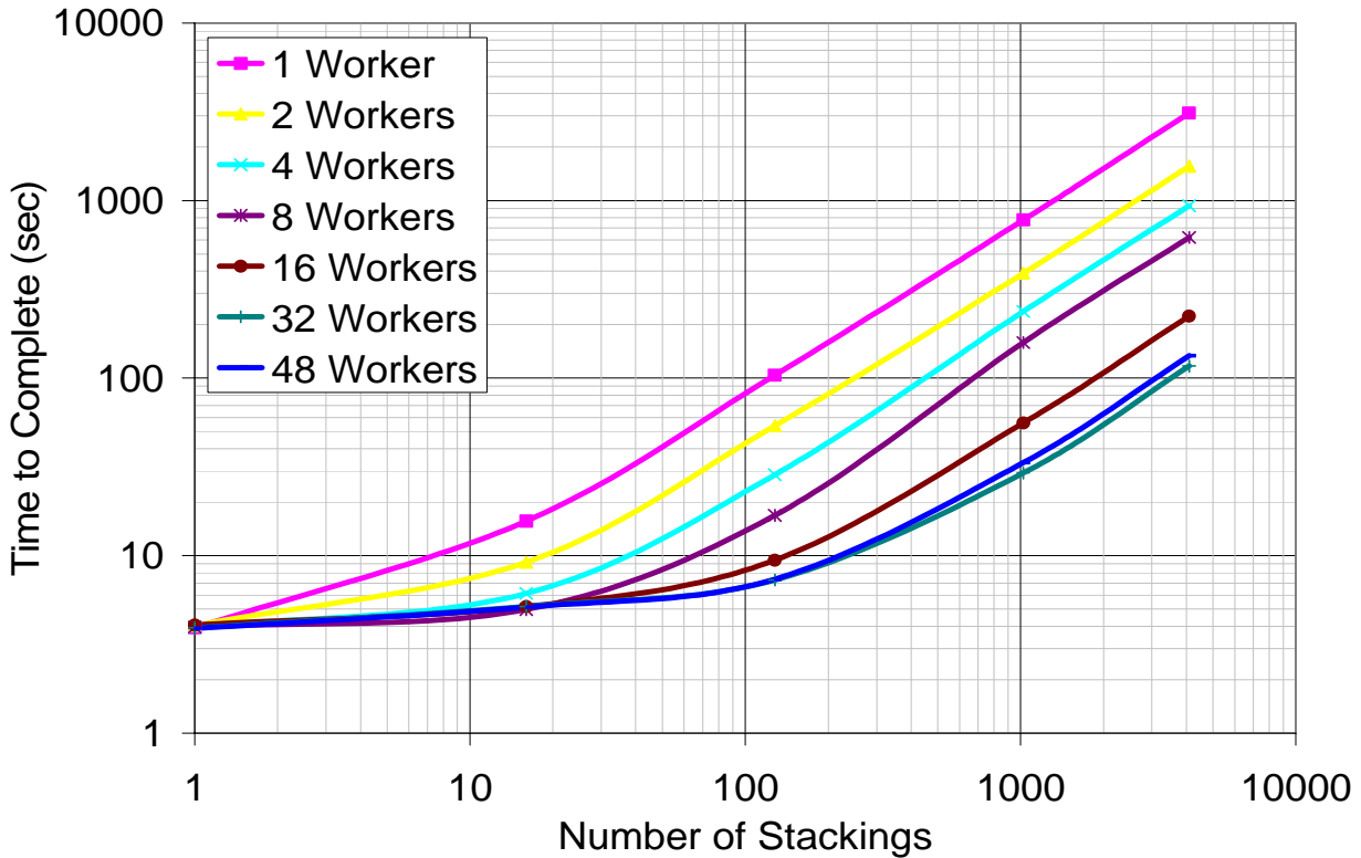
Figure 5: Stacking Performance on compressed images on the ANL GPFS
